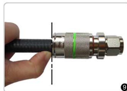
9 Screw the connector onto the cable until it reaches the marked line. Over tighten is forbidden.
