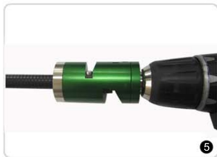
5 Insert the cable into the trimming tool. Select the low speed on the drill or 400~600 RPM on a variable speed drill. Trim the cable until no further debris generated.
